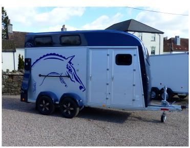
Unique design and generous space configuration: The new Big Portax with an interior width of 1850 mm and an internal height of 2400 mm provides even more space for you and your horses. The standard features include the world-class 'WCFplus' chassis to automotive standard and a large tack room that is separated from the horse compartment by a partition wall with a height of 2100 mm.
