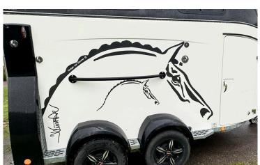
High class: With an internal length of 3900 mm and an internal width of 1750 mm, the Grand Master SR places special emphasis on a large space and a great design. The trailer has exclusive features such as LED interior lighting switchable from white to blue, aluminium rims, sliding windows and a roof vent. Special highlights are the variable centre post partition wall and the walk-in saddle room, which is accessible from the inside through a man-high door
