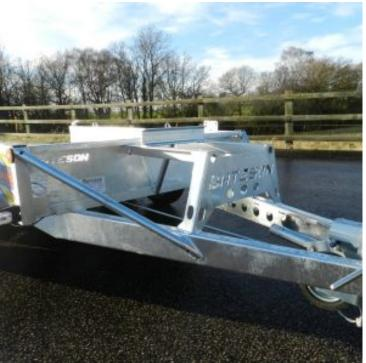
2600kg Mini Excavator trailer for machines up to 2100kg Model 26MD is a trailer designed to transport a Mini Excavator up to 2100kg. or a 1.5 ton excavator with extra buckets and equipment. It is fabricated with a heavy duty hot dipped galvanised steel chassis with integral welded steel treadplate mudguards suitable for standing on.Extended draw bar and high bucket carrier allows the digger boom to have a good clearance from back of vehicles
