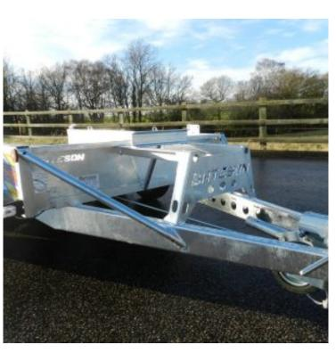
2600kg Mini Excavator trailer for machines up to 2100kg Model 26MD is a trailer designed to transport a Mini Excavator up to 2100kg. or a 1.5 ton excavator with extra buckets and equipment. It is fabricated with a heavy duty hot dipped galvanised steel chassis with integral welded steel treadplate mudguards suitable for standing on. Extended draw bar and high bucket carrier allows the digger boom to have a good clearance from back of vehicles
