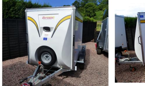
8' x 4' x 5' Lightweight twin axle van trailer The 160V is the smallest trailer with brakes, with twin axles and 10" wheels it provides a very smooth ride, ideal for use with medium size cars.Standard equipment includes a locking coupling, spare wheel and carrier, and our ingenious coupling mirror, which allows the hitch to be seen during coupling to eliminate misalignment and damaged bumpers
