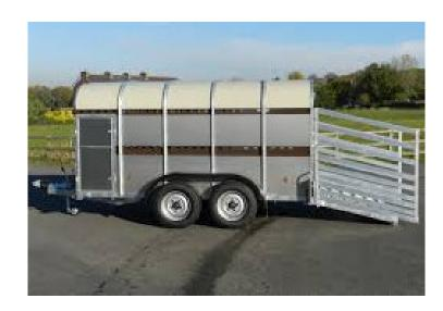
Model 48LT is a our largest Livestock Trailer fitted with Land Rover size 16" wheels. We do not make larger models for safety and legal reasons. This trailer loaded with livestock could exceed the 3500kg maximum gross weight that can be towed by a 4 x4. A larger trailer, particularly if fitted with three axles, would weigh much more and would have a corresponding reduction in payload.
