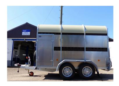
8' x 5' x 6' Livestock Trailer for use with cars and light vehicles. Model 30LT is the smallest trailer in our Livestock Trailers range that will accommodate two cattle. It is It is lightweight and ideal for use with cars or smaller towing vehicles.
