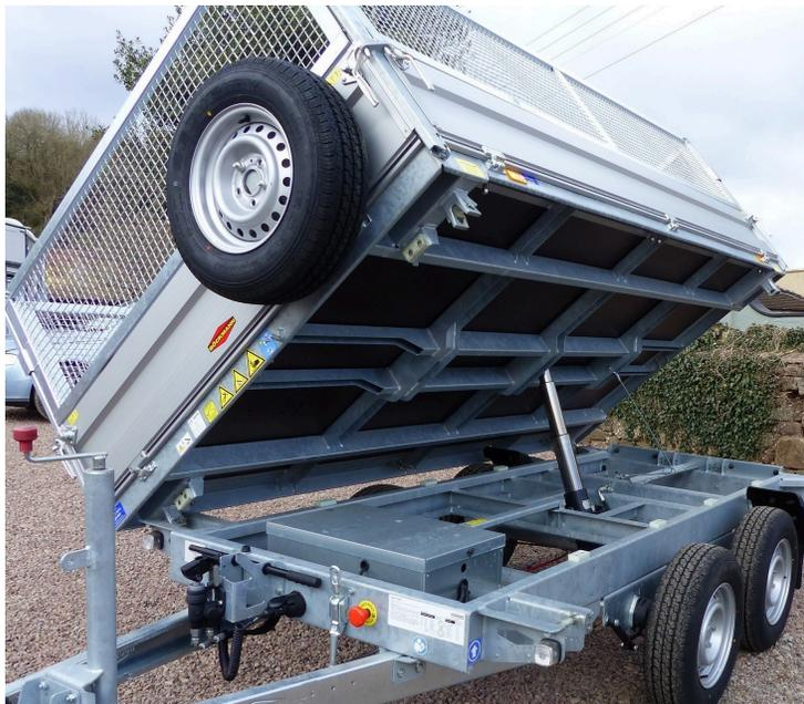
The three-way tippers in the professional version are vehicles of absolute professional quality and equipment. They impress with a solid and robust construction, an impressive 45 ° tilt angle and a countersunk lashing bracket system.
