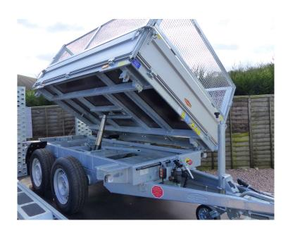
The three-way tippers in the professional version are vehicles of absolute professional quality and equipment. They impress with a solid and robust construction, an impressive  $45^{\circ}$  tilt angle and a countersunk lashing bracket system.
